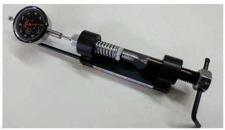
Tester set up for testing a bullet.
